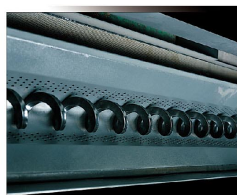
Automatic chip removal (Screw type chip conveyor)
