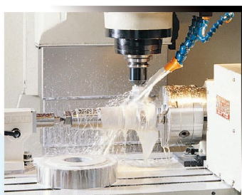
High pressure coolant (P:3.5 kg/cm 2 , Q:100 l/min)
