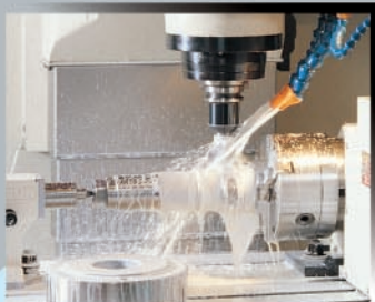
High Pressure Coolant (P:3.5 kg/cm 2 , Q:100 l/min)
